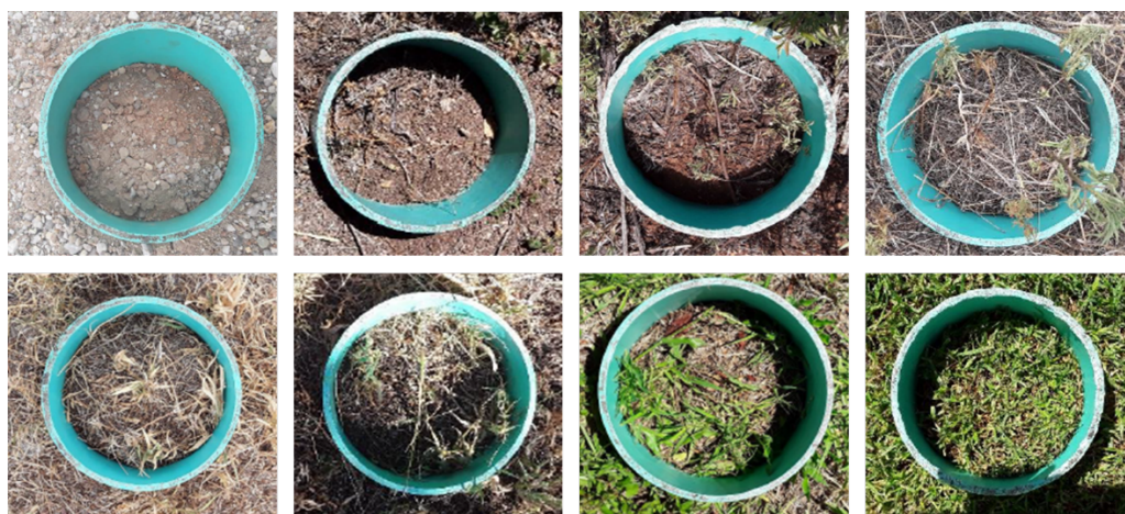
Figure E15: Variability in vegetative surface cover illustrates complexity in background correction of DCC data in real-time.
