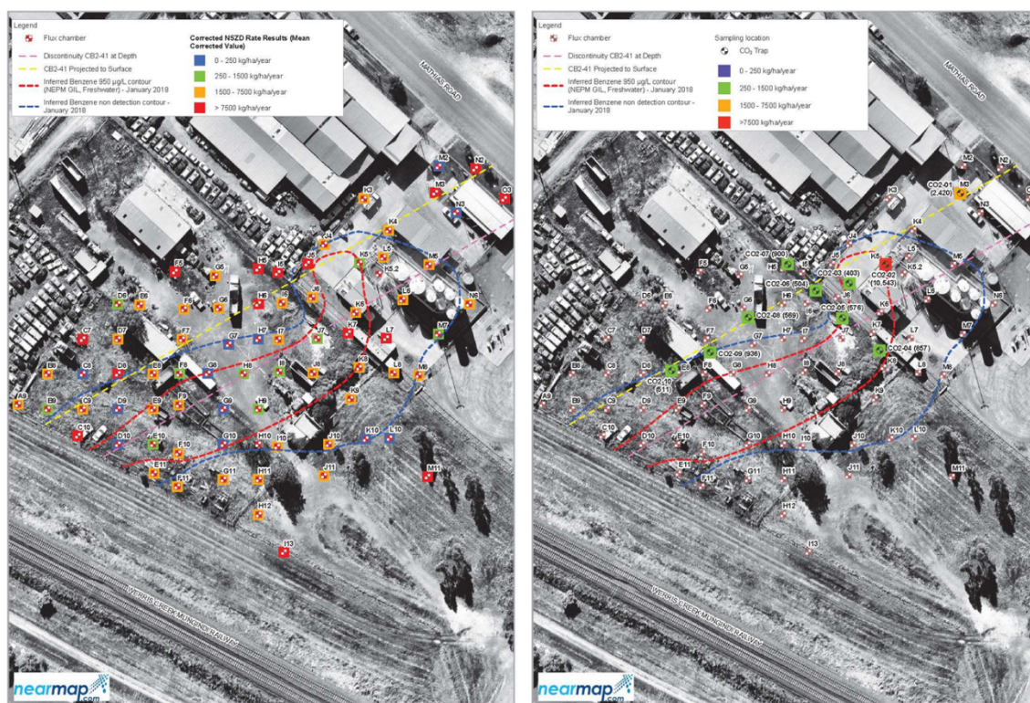
Figure E14: NSZD estimates based on DCC (left) and CO 2 Trap (right) results
