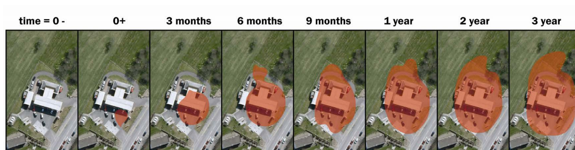
Figure 4: LNAPL release of fuel oil observed in monitoring wells showing that LNAPL body stability was largely achieved in 1 year (API 2004)
