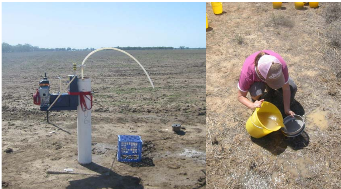
Figure 2. An inertia pump set up for groundwater extraction - filtering groundwater samples after pumping to collect stygofauna.
