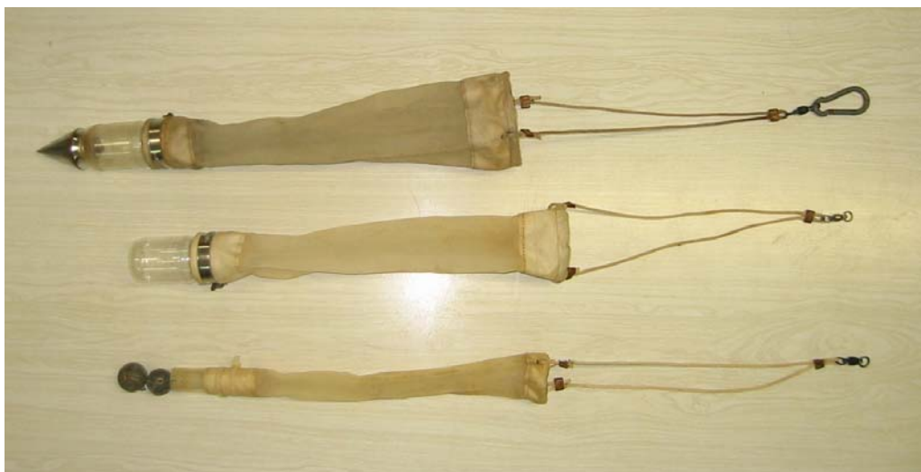
Figure 1. Weighted plankton nests of various diameters and mesh sizes used for sampling stygofauna.
